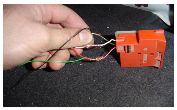
(5) Turn on the ignition and wait for about 60 seconds. Look at the dashboard. Still on SRS light. It stays on because it was not properly connected signal cable.
