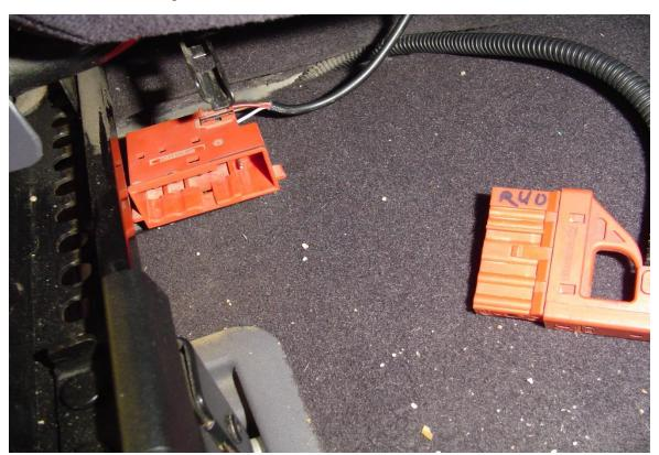
(3) Cut the sensor cable for you in a convenient location
