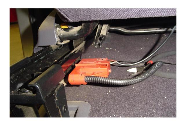
(2) Switch off the ignition and disconnect the connector. ,
