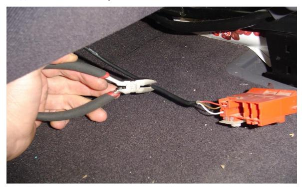
(4) Connect the emulator and connector cables and the corresponding order: signal wire connect with the signal wire; grounding wire to the grounding wire; plus wire to the plus wire. Green (function) wire connect the plus wire or earth wire, this is how you carried out the emulator adaptation. Eg. This time it is connected to the plus wire.
